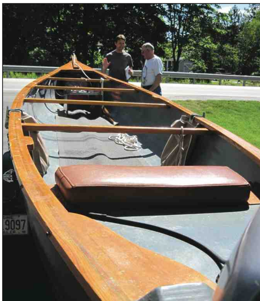
Figure 5. The interior of Claude's 22-foot Grand Laker canoe. Claude modified the classic design with a fiberglass interior, ash trim, and a casting platform in the stern.
