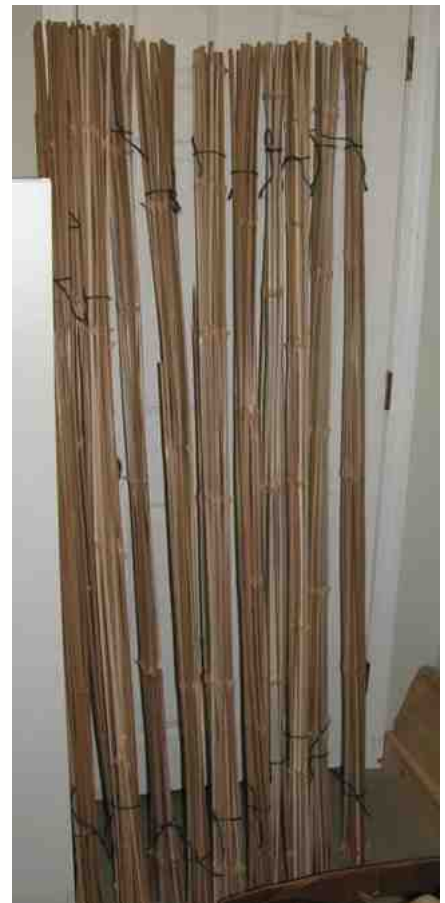
Bamboo strips in Steve Campbell’s workshop, ready for node filing and milling.
