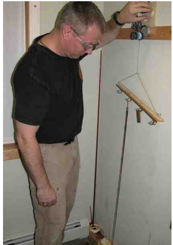
Steve Campbell operating a motorized rod lifter at a varnish dip tank (similar to what Sam Carlson used).
