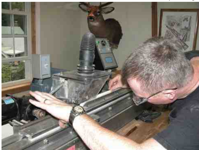
Steve Campbell setting up the milling machine to run a bamboo strip through.
