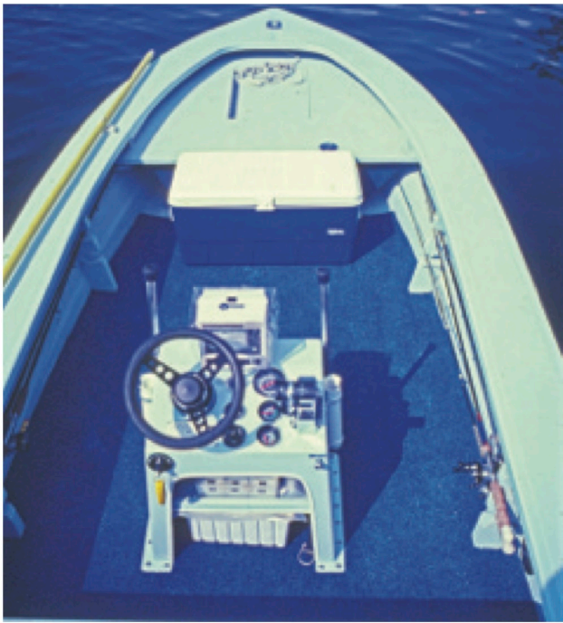
The interior of the author's Hewes Redfisher, built in 1976. It had no inner liner or built-in storage containers, and the otherwise bare cockpit floor was covered with outdoor carpet to reduce noise.
