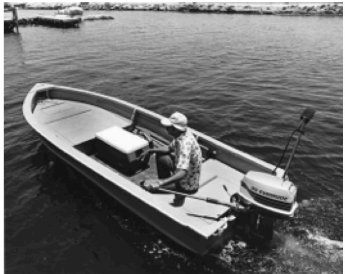
In the Alum2, the middle seat (second seat forward from the transom) has been removed to create an open cockpit. The two front seats are spanned with ½-inch marine plywood to create a spacious forward casting platform; the rear platform is created in the same manner.
