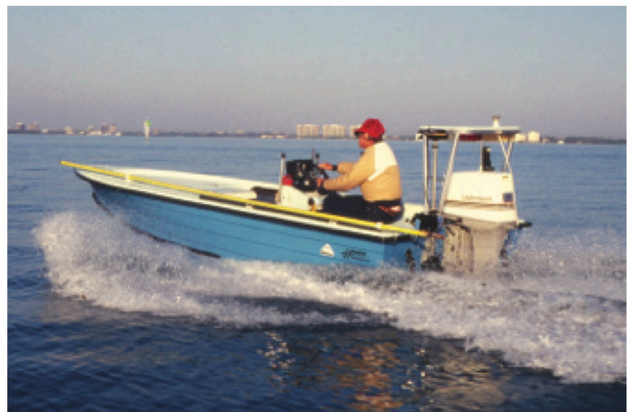
The 1984 16-foot Kevlar version of the Hewes Bonefisher, with Bob Hewes at the helm. Note the elevated poling platform on the transom.
