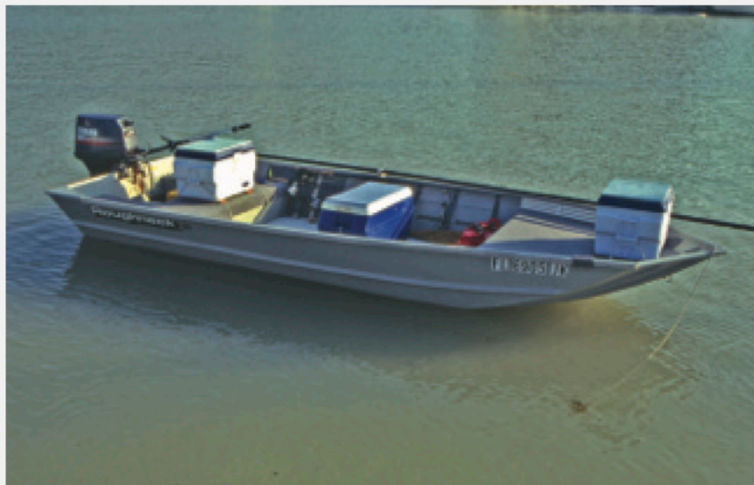
A 16-foot aluminum jon boat built up in the same manner as the Alum2 skiff. Modified coolers are used for both storage and as elevated platforms for better visibility.
