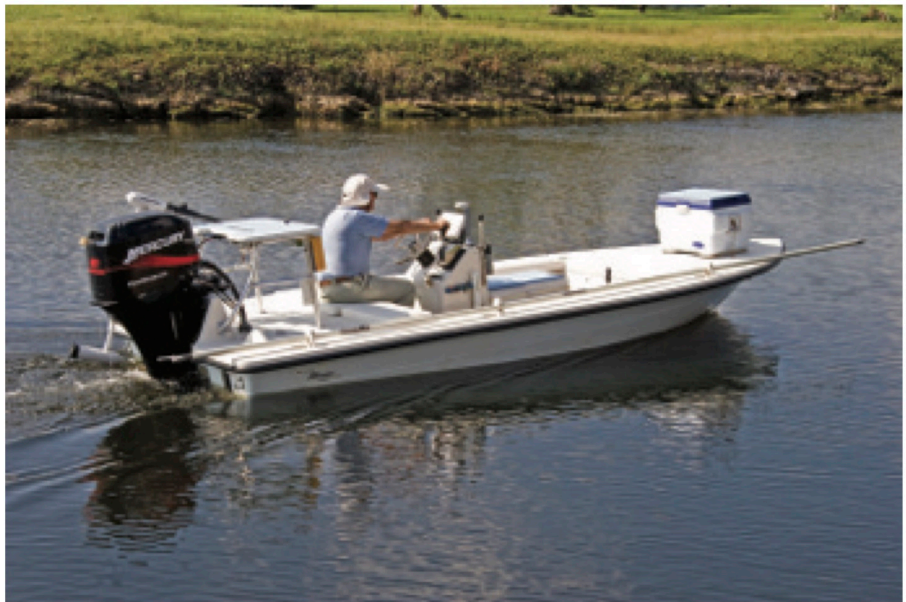
An ultralightweight 17-foot flats skiff with a tunnel hull. It is built using Kevlar carbon layers with foam in between and floats in less than 6 inches of water with two anglers aboard.
