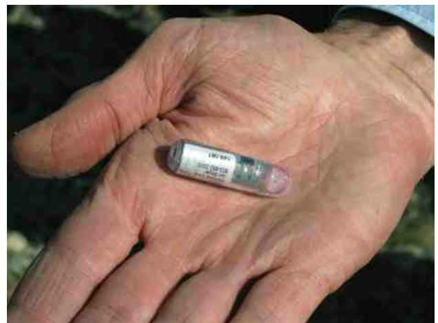
Adult whitefish were surgically implanted with these radio transmitters to track their movements over a period of two years, beginning in the spring of 2012.
