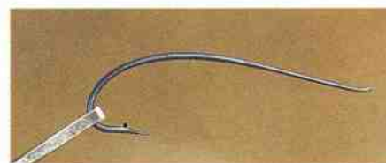
A fully functional hook made by the author. The blue color indicates the temperature at which the steel was tempered.
