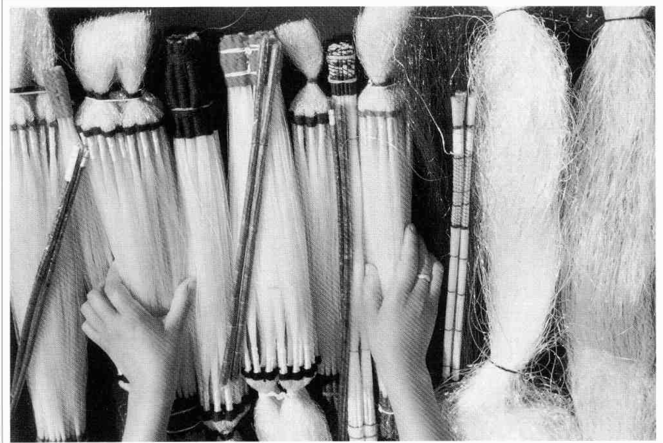
The yarn-wrapped hanks of silk gut were straightened, sorted, polished, and trimmed to ready them for commercial sale to tackle companies and medical suppliers. These 36,000 strands of gut are the products of 18,000 silkworms. Photograph by Luis Marden © National Geographic Society.
